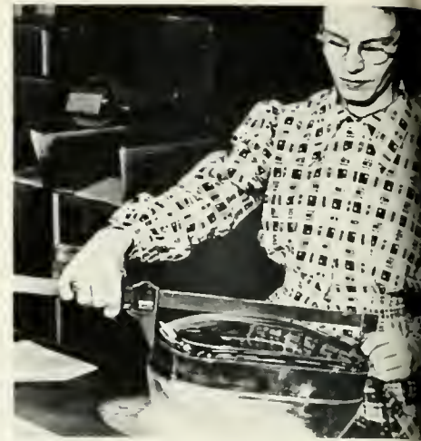
Manufacturing process begins with inspection of all parts comprising the tube, whether glass or metal-shell type.
