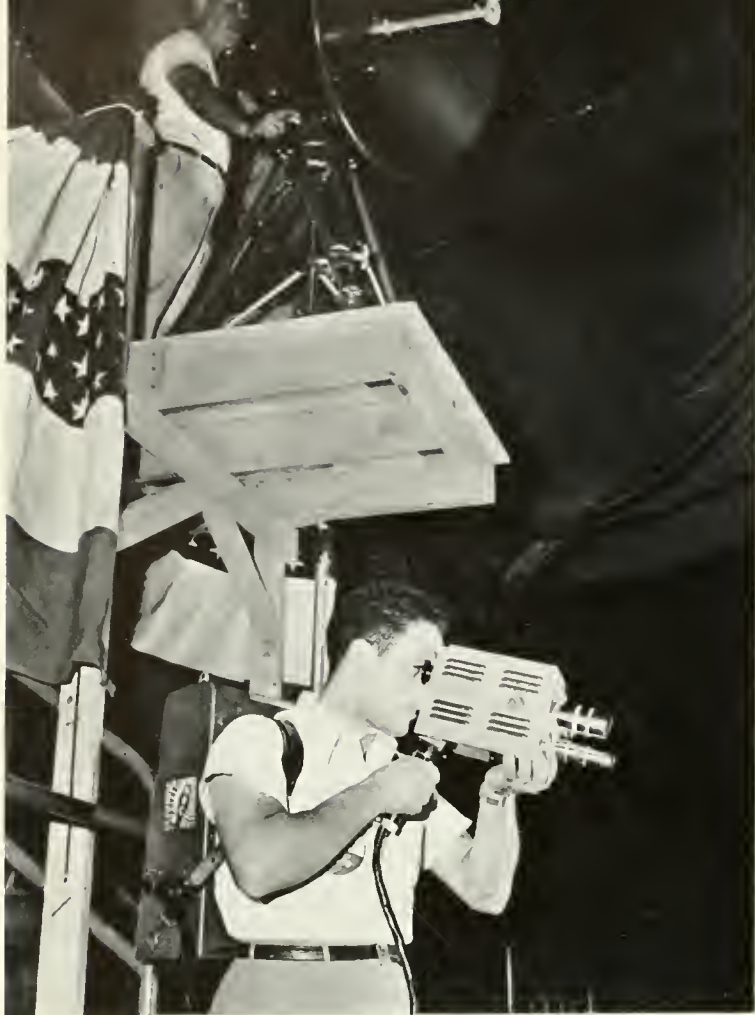
Portable walkie-lookie unit is dwarfed by a huge parabolic receiving unit used to pick up microwave signals from walkie-talkies on the auditorium floor.
