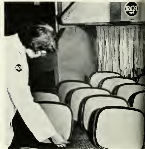
Kinescopes are baked in huge ovens to "bail" out impurities and to dry the inside graphite coating.
